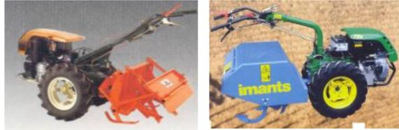
Secondary tillage tools like power harrows break clods left by primary tillage tools or flatten seed beds, breakup crusts and incorporate soil amendments or bury stones or debris and generally finish a seedbed.
