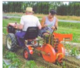
Once crop is growing an interrow cultivator can be used with a walking tractor - to clean weeds on either side of growing row.
