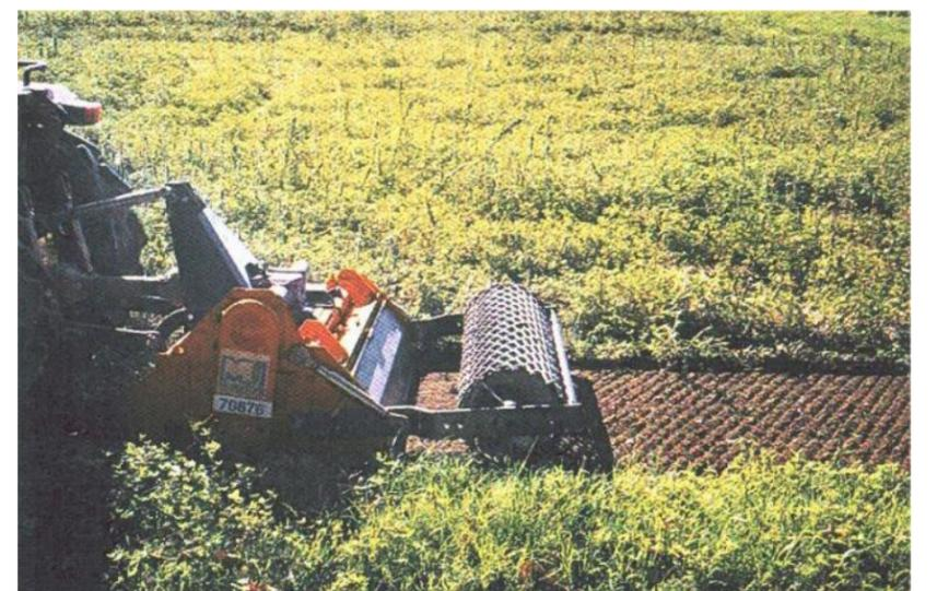
wide ready to plant bed is created. With the smallest of the Hydrostatic four wheel tractors a 33" bed is prepared in one pass. With a 30 HP tractor you could use a stone/burying tiller that simultaneously creates a raised bed with 33" bed top.
