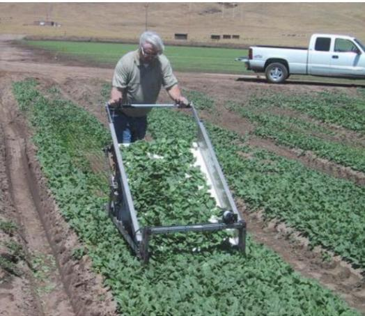
In its simplest form, machine is pushed by operator just as you would a push type lawn mower. Two bed-width rollers carry weight of machine with front roller controlling cutting height and rear roller supporting weight of machine and crop. Operator controls rate of advance to meet crop density and to insure
