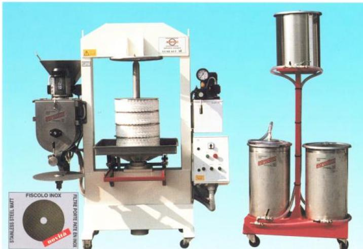
Here is an ultra modern press using hydraulic pressure and electronic controls to keep constant pressure as oil begins to run out of paste.
