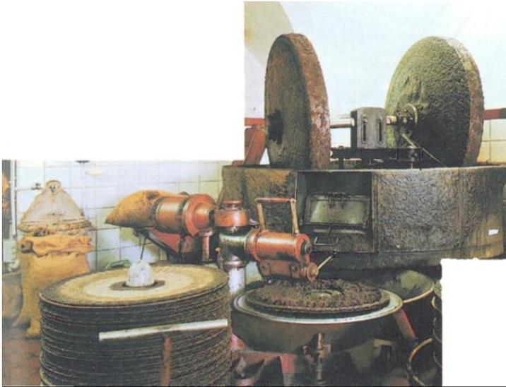
Pictured here is a traditional stone Arastra that was electrified in early 1900's and continues in use to this day. Note the dosing machine spreading Olive paste onto mats ready to be carried to vertical press.
