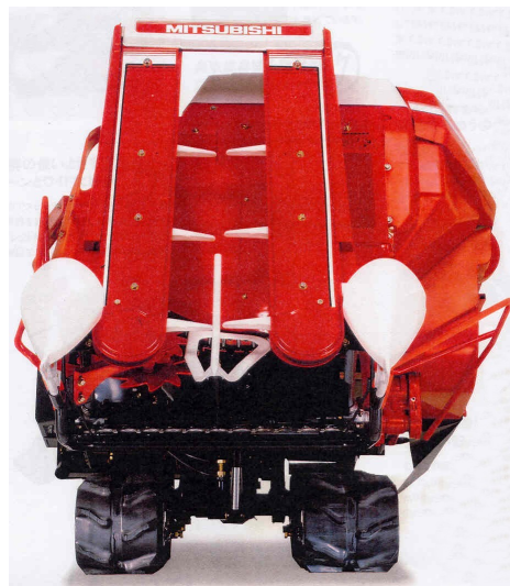
#2 Because the crawler width is smaller than the reaping width, any kind of reap- ing is possible. Unique forced pulling system makes any leaned crop to be reaped.
