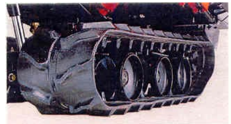
#3 Wide crawler Safe travelling on any kind of field con- dition, especially on wet field.
