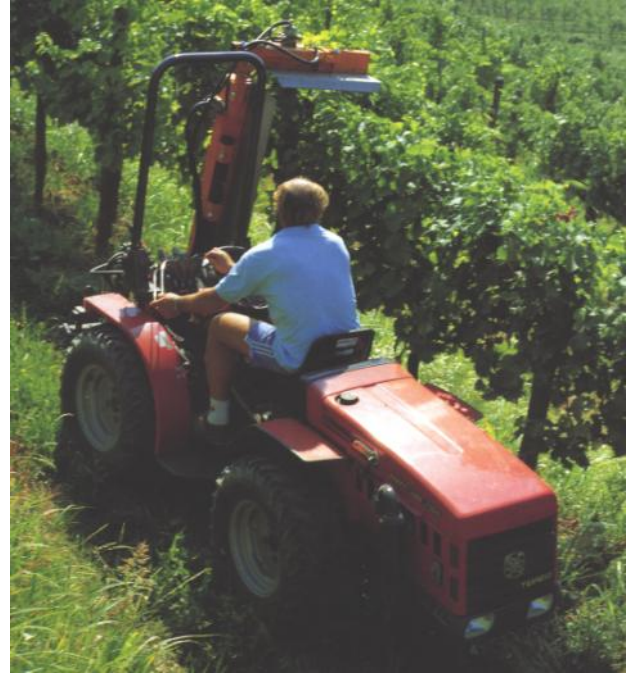
In this picture a vineyard hedging tool is shaping vines, the tractor is an Antonio Carraro articulated Vigneto model.
