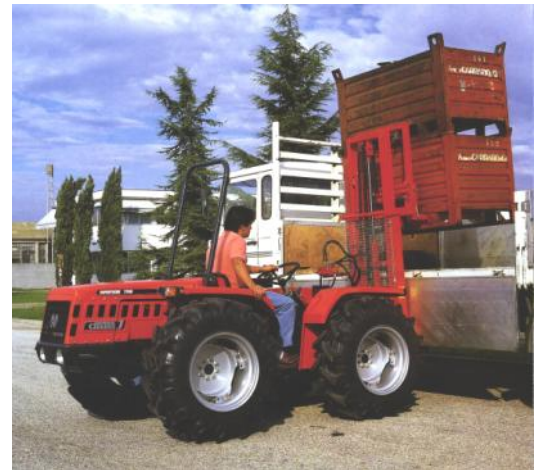
Forklift mast allows handling of pallets and bins with precision and safety. Tractor shown is articulated 60 HP Antonio Carraro Supertigre 7700.
