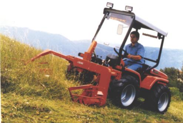
Pictured here is 6 ft. wide double acting sicklebar mower being used to swath hay. Tractor is Antonio Carraro TTR3800 hydrostatic reversible tractor. This style of sicklebar is less prone to plug in damp or viney crops.
