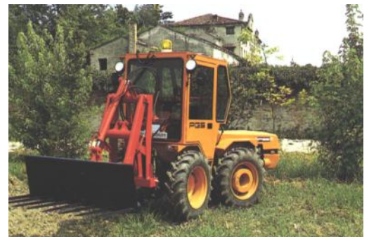
Skip Loader function can be performed by adding rear loader and reversing tractor lifts loose material up to eight feet to load trucks or spreaders or can be used to turn compost piles etc. Some versions of this type of loader mount to brackets on tractors axles and some mount on 3 pt.
