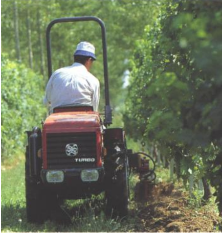
A vineyard grape hoe that tills berm area is ideally mounted in front of driver, pictured here on reversed Antonio Carraro 5500 Vigneto.
