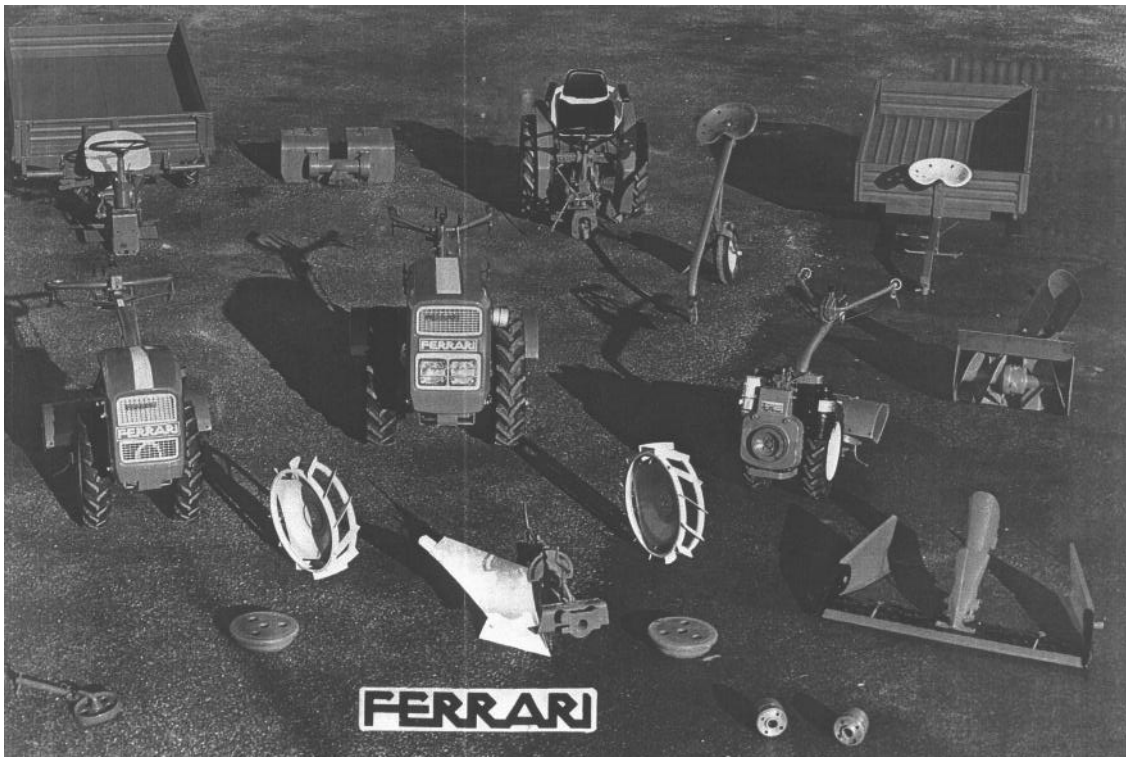
1971 Dealer display showing model 94 walking tractor in center and rear assembly to right and behind it. The driven axle trailer could also combine with walking tractor to form a transporter, another unique variation.
