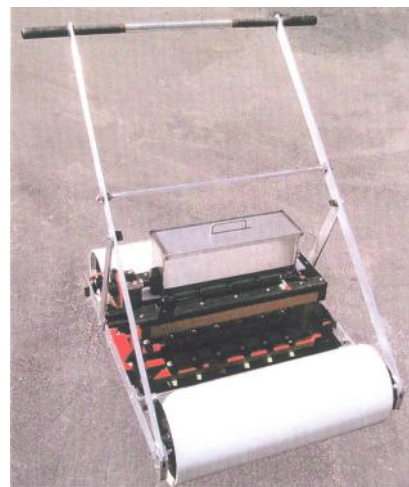
Inside seed box rotating brushes sweep seed into opener.
