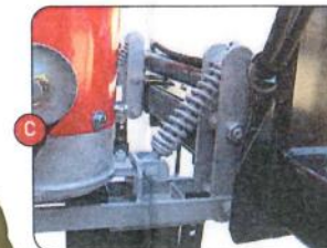
E. Shock absorbing springs. Each body is equipped with a separate shock absorbing spring in order to thus safely overcome the irregularities and foreign bodies in the ground.
