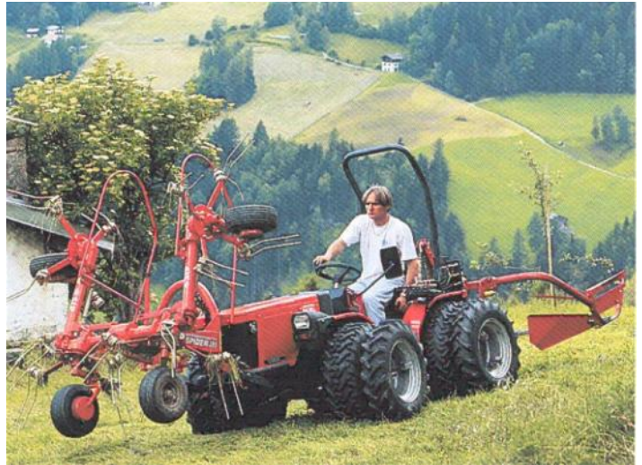
Bidirectional TTR 4400 with double acting cycle bar on rear 3 pt and gyro rake on front 3 pt. in transport mode.
