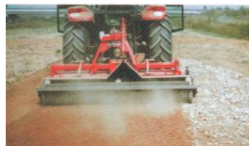
One pass, Stone/debris burying, bed making Tiller
