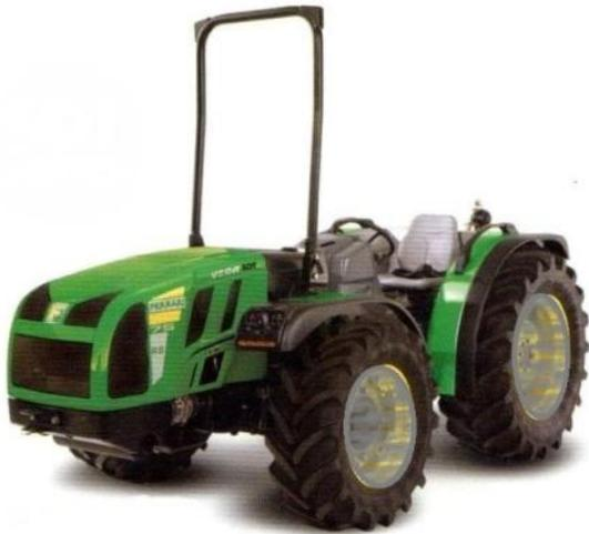
The Vega SDT is an ultra low profile mono-directional tractor 67, 83, or 91 HP that uses slightly smaller diameter front drive wheels that can be engaged or disengaged to allow it to minimize soil disturbance on very tight turns and to allow 24 miles per hour on road. The SDT low center of gravity allows side slope performance generally achieved only by crawlers. This 4900 lb. tractor can also be equipped with a front 3pt., lifting 1700lbs.
