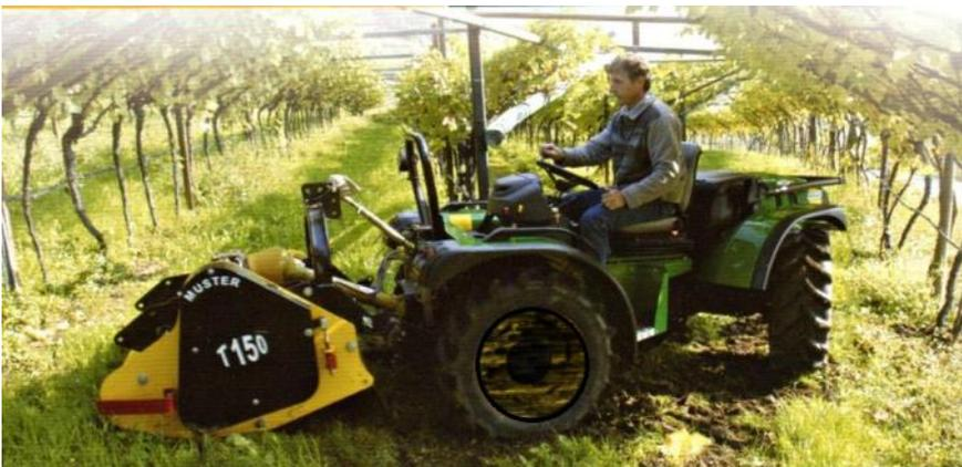
Both styles of Ferrari Dualsteer models share same 4 wheel in-board wet disc brakes, push button engagement of PTO via wet multi-disc clutch and 16 ground speeds forward and 16 reverse ground speeds and 15 degrees of longitudinal oscillation to keep all 4 wheels engaging rough terrain.
