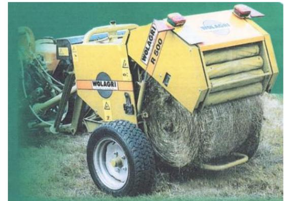
The smaller scale producer can instead use a small round baler with a net wrap option to pick bean material from windrow to form small round bales that are easy to handle and store. The net wrap helps to retain beans until you have time to put them through a stationary thresher. These balers come in sizes powered by 15 plus HP tractors.
