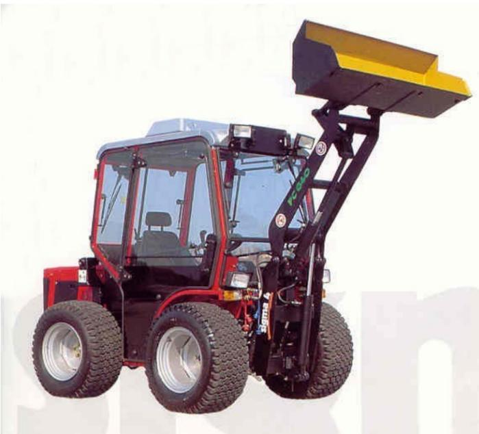
This same model loader was originally designed specifically for Antonio Carraro's hydrostatic tractor model Sp 4400 and HST 4400 (38 HP). Loader has a hydraulic jack stand so that mounting and demounting loader is easily done by operators without strain and requires no tools.
