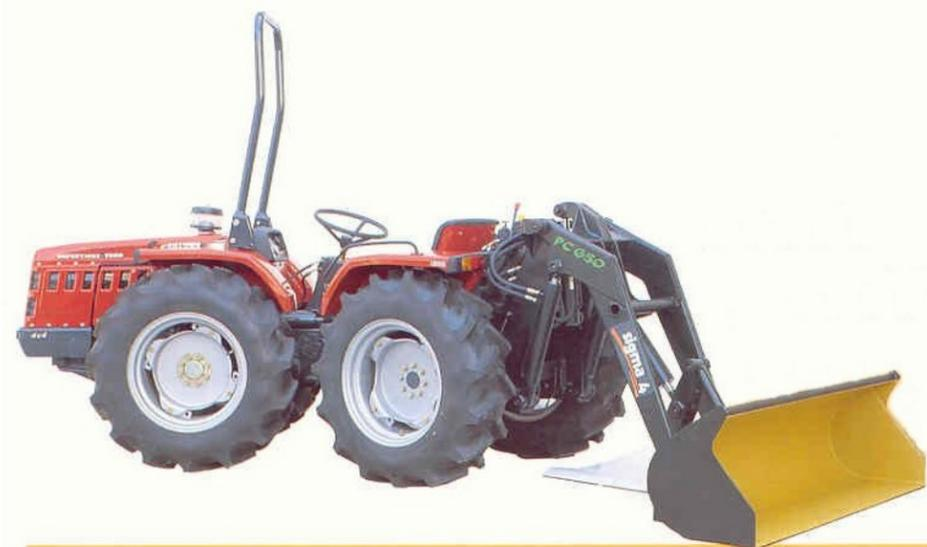
A large version of this loader, model 650, is designed for 60 plus HP tractors and mounts to same brackets attached to rear axle of the tractor mounting and demounting is done the same way as the smaller version.
