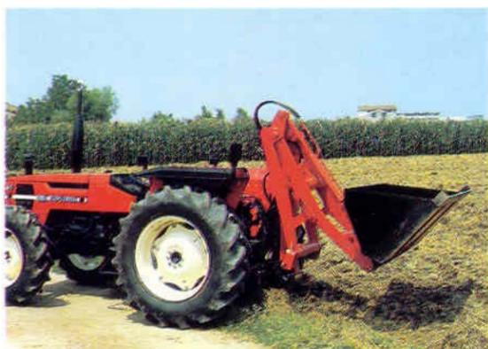
Still another rear loader manufacturer uses the tractors 3 pt arms to support the entire loader. A hydraulic top link allows loader mast to be tilted to bring load in closer to tractor. Nomag makes 6 models to fit 20 to 130 HP tractors.
