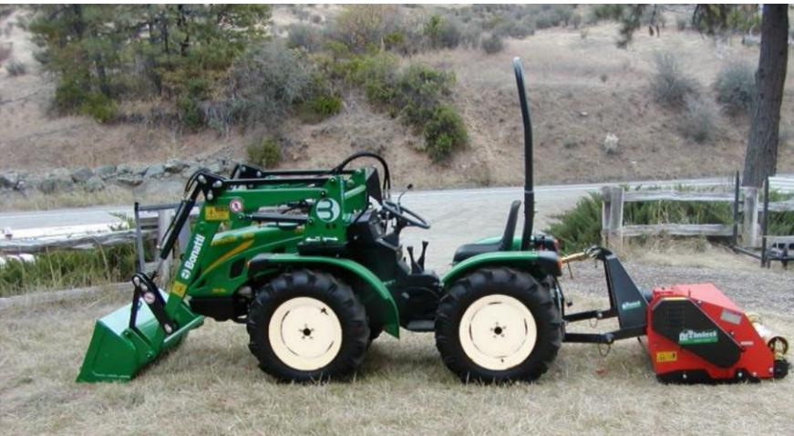
Ferrari offers the bidirectional option in its mid range Cobram models of 35 HP and 46 HP both in conventional steering and articulated models. Articulated models are especially suited to the bidirectional mode of operation because steering behavior is identical whether you face engine end or face 3 pt. end of tractor, the rear wheels follow
