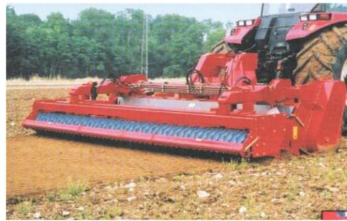
tines. Soil, fine, free of debris, pass through while stones, root clumps and other debris fall to the bottom of the cut and are buried by clean soil. Mesh roller firms soil and leaves it uniformly flat.
