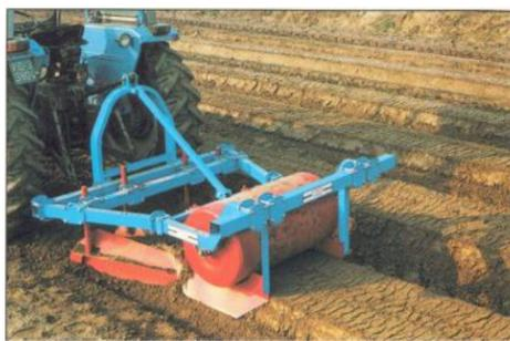
When one wants to prepare fine seed beds from 39" on up in width the answer is a powered bed maker. The Falc Cultiline is an example and one that uses a unique spiked rotor that breaks up
