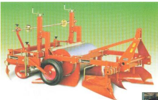
The European passive bed shapers generally add a roller to flatten and consolidate the bed top. With most of the passive bed shapers, bed tops range up to about 35" wide.
