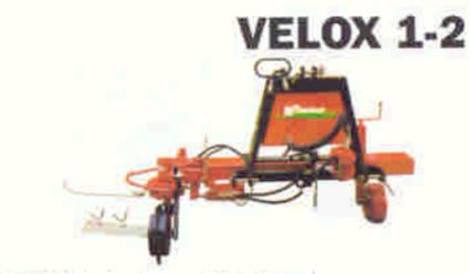
When maintaining grass row center is the choice there are several more options for inrow tillage, including hoes, plows and discs. The hoe consists of a cutting blade that undercuts weeds working just a few inches below the berm surface and a sensor system to rotate blade out of the row to avoid contact with crop plant. The horizontal blade can be replaced by a moldboard plow that pulls dirt away from berm and away from crop plant.
