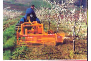
A somewhat more recent development is the offsetting power harrow that uses tines rotating on vertical axis. As with the rototiller these can be designed to do narrow bands or wide enough to do much of the row centers in each pass.
