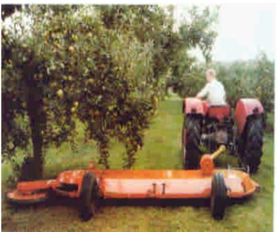
In these the outrigger is usually a rotary mower driven by a belt or hydraulic motor and mounted on an arm that is spring loaded. A rubber bumper on the blade guard comes in contact with the trunk of the crop plant causing the outrigger to move out and around the plant. Once the blade guard, that protected plant trunk from being damaged, is no longer in contact the spring in the arm pushes the outrigger out to mow the berm area between the crop plants.
