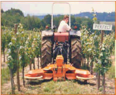
The first group are mowers designed to keep compatible covers crops clipped short to deny weed varieties a chance establishing themselves in significant numbers, and to prevent them from maturing and going to seed. The simplest form is an outrigger mounted on the side of a mower used to mow the centers.
