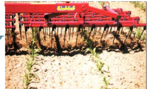
16A Rod weeder : spring steel tines pull out shallow rooted weeds.
