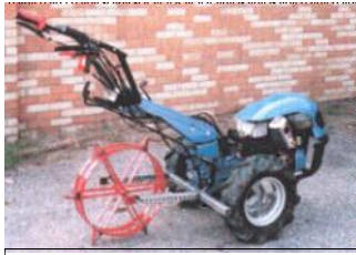
1B Dibble wheel pokes holes into plastic for planting. Open concept allows easy spacing changes and spike changes for different sized plugs.
