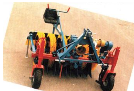
21 Brush Hoe uses stiff bristled brushes to "sweep" out weeds while metal tunnels protect crop.
