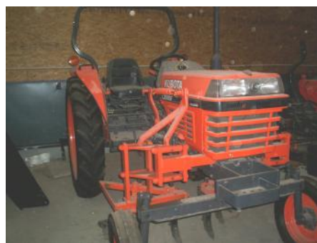
22 Standard Kubota L3000 with front and rear axles lengthened on right so driver can see belly mounted cultivator.
