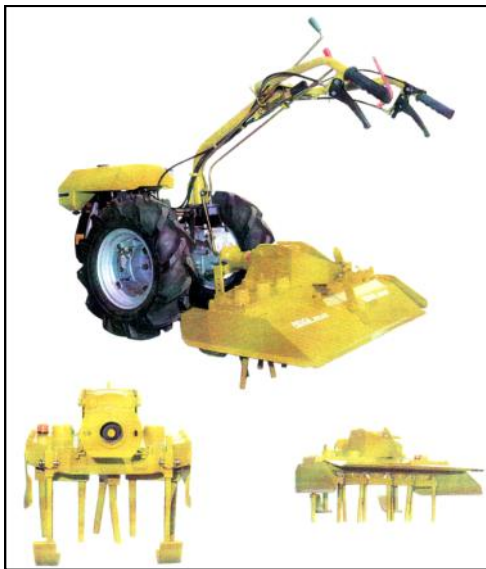
12 Narrow Power Harrow takes out weeds between growing rows. note depth control skids
