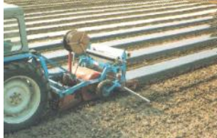
2 One of the many bed-formers that combine a mulch layer for one pass operation. Note drip tape also laid.
