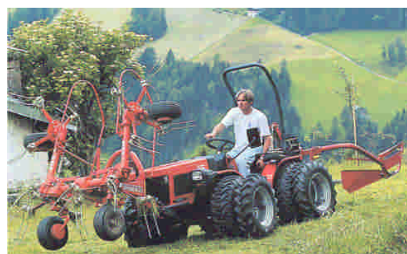
Note small multiple Gyros mounted on front of Bidirectional Tractor. Note Center mounted double cyclebar mower on rear 3 pt.
