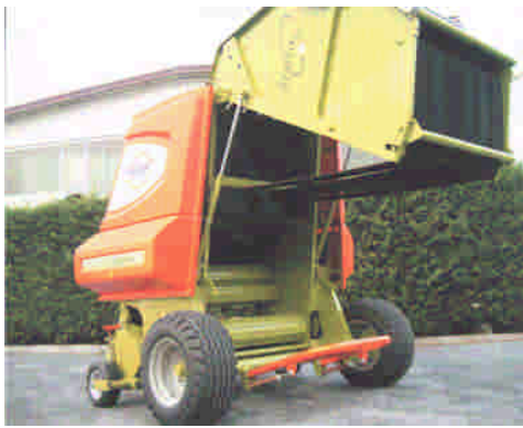
Belt type makes bales 32" - 65" diameter, loose or high density.
