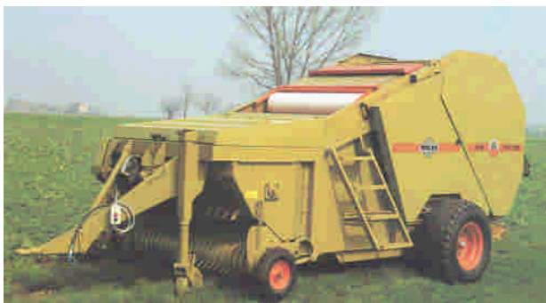
Fixed bale size but 2nd bale is started before 1st bale is discharged for continuous run.
