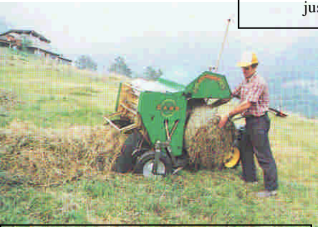
Baler for walking tractor just 12 HP needed.
