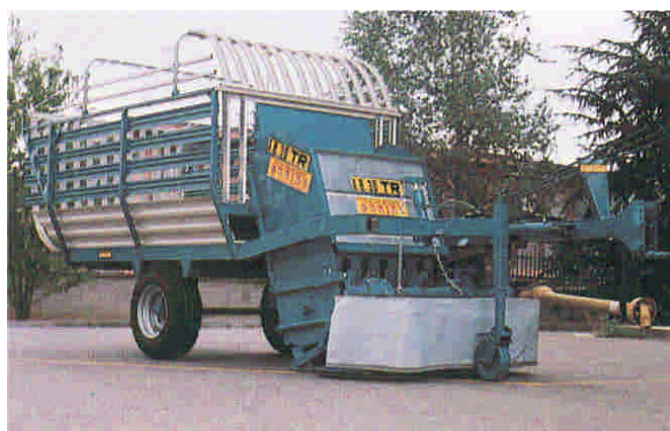
Forage is cut with drum mower and then lifted into wagon
