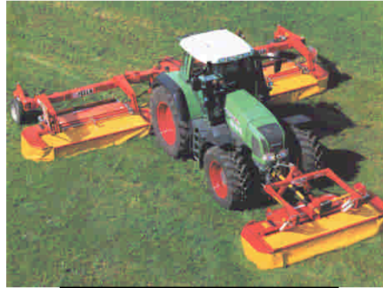
Disc mowers set up for maximum cut-
