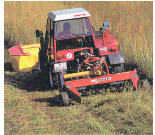
Front drum mower with rear conditioner distributes weight equally.
