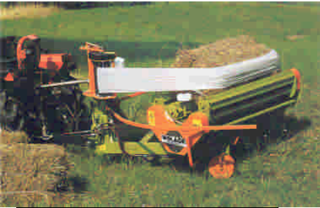
Bale wrapper for 20 HP Tractors does round or square bales.
